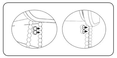
**Upper Limit**, pull the back chain until the desired upper position. Then, snap the chain stop to the bead just below the clutch.
