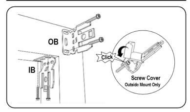
Secure the roller shade installation brackets with the supplied screws. If shade was ordered as outside mount (OB), attach the supplied screw covers on to the bracket for a finished look.
