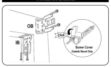
Secure the roller shade installation brackets with the supplied screws. If shade was ordered as outside mount (OB), attach the supplied screw covers on to the bracket for a finished look.
