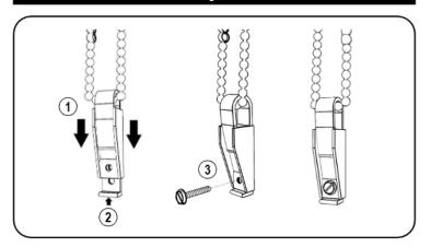
Slide device down to the bottom of the bead chain and pull down until the chain is taut on both sides. Mark the screw hole and install the device with the screws provided.
