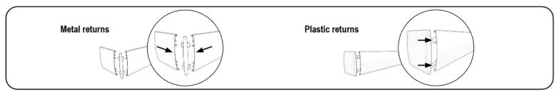
Metal returns (Outside mount only) include a plastic corner connector. Plastic returns (Inside mount with Outside Mounted fascia) snap on the end of the fascia.
